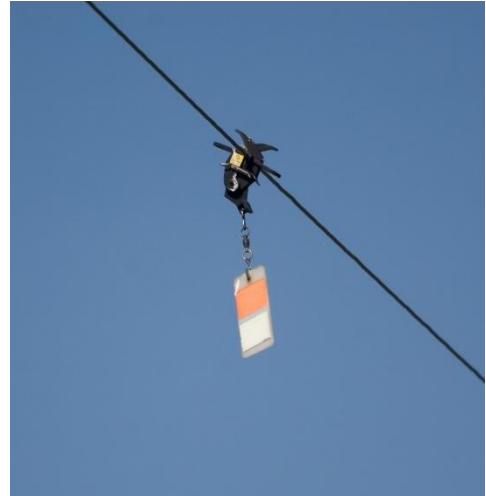
Figure 24B. Several years after deployment the line markers used to experimentally test whether line collisions could be reduced for sandhill crane and other birds (Yee 2007) were broken, twisted and missing due to exposure to sun, rain and wind. Durability is an issue. Photo by Shawn Smallwood.
